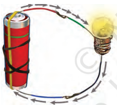
Fig.9.6 Direction of current in an electric circuit
